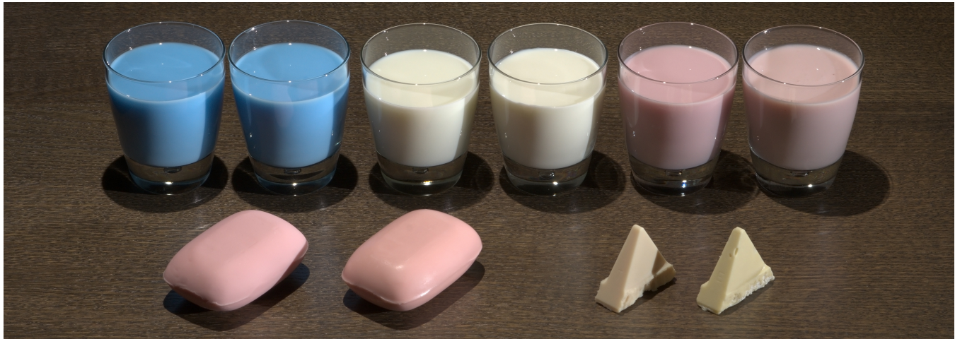
Figure 1: A side by side comparison of real translucent materials (right) next to their silicone replicas (left) fabricated using our method.
